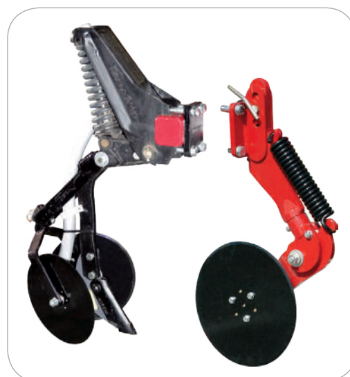
▲ An opener with a shank and leveling wheels (left); A cutting disc (right) - optional
